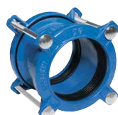
Series 601 Supa® straight coupling universal for uPVC, AC, steel, cast iron and ductile iron pipes Ductile iron DN40-400 PN16
